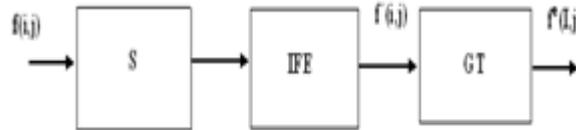
**Figure 2: Block Diagram of the Generalized Image Enhancement System**
